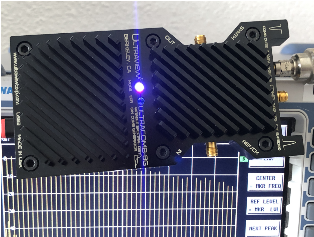
Fig 3. Ultracom-B-8G generating comb with 200MHz-spaced pickets, with 0dBm amplitudes to 3GHz, -3dBm at 5.4GHz and -11dBm at 8GHz and -18dBm at 10GHz.
