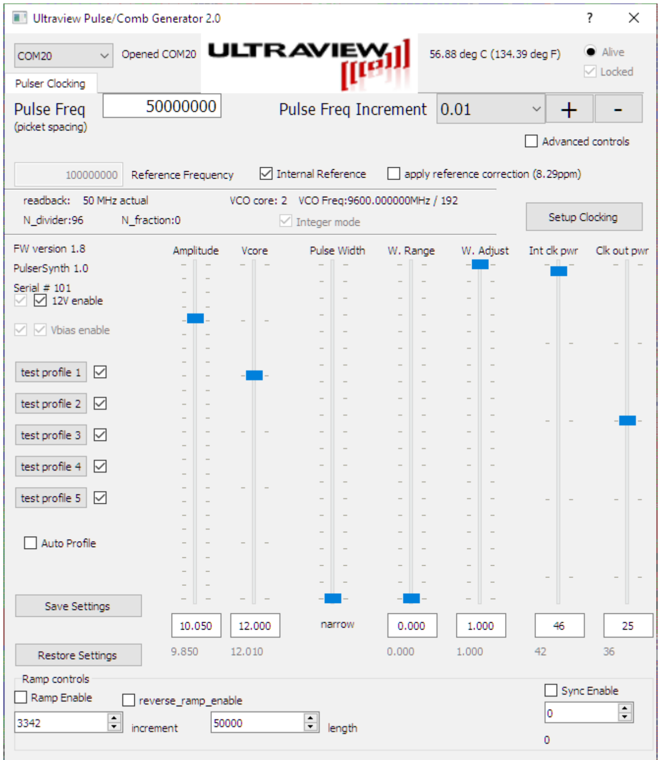
Figure 1. Default settings for fastest pulses. Be sure to select the appropriate COM port in the upper left and make sure the 'Alive' indicator is flashing and a temperature is being displayed. Then click “Restore Settings” to set unit to default or last programmed settings.
